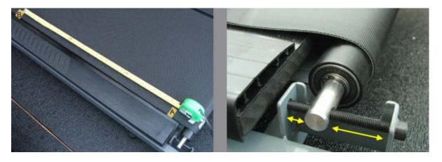
Another method would be to fully remove the existing Running Belt form the Treadmill but leaving the Front Drive Roller securely in place and then set the Rear Slave Roller in a position based on about just before half way or mid way (30%) of the Belt Adjustment bolt thread (also known as Tension/Tracking bolts). With Rollers in position measure completely around the Front and Rear Rollers for an accurate measurement
